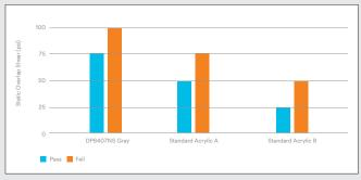
Chart shows the shear load (dead load in shear) that the adhesive can hold at 400°F (powder coat temperature). Blue bar: load held. Orange bar: load did not hold (fail). DP8407NS can hold a dead load in shear of 75 lbs during a powder coat cycle; but may fail at higher loads.
