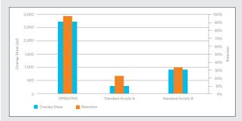
On abraded, cold rolled steel, DP8407NS shows high shear strength after exposure to 150°F and 80% relative humidity for 500 hours (accelerated outdoor weathering), whereas some competitive acrylics will lose strength due to steel corrosion accelerated by the adhesive.
