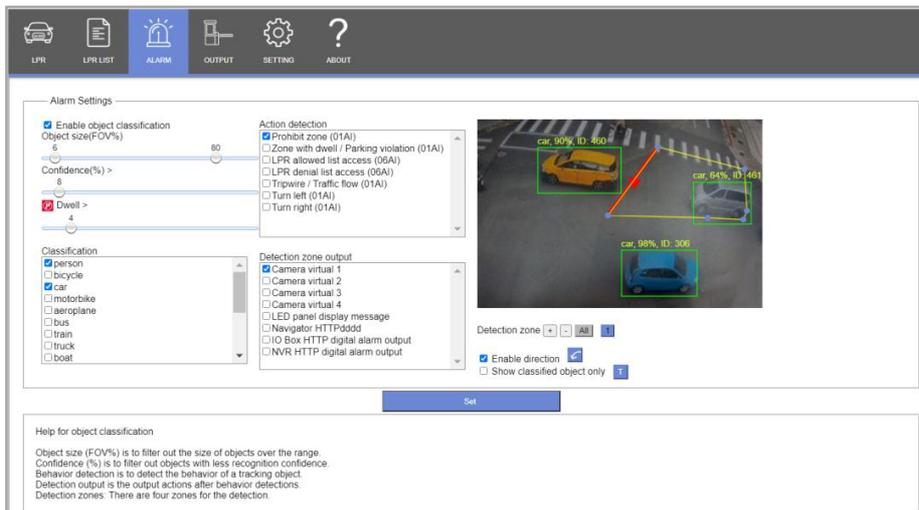
**Note:** It is important to disable “Enable object classification” feature, if object detection is not used.
