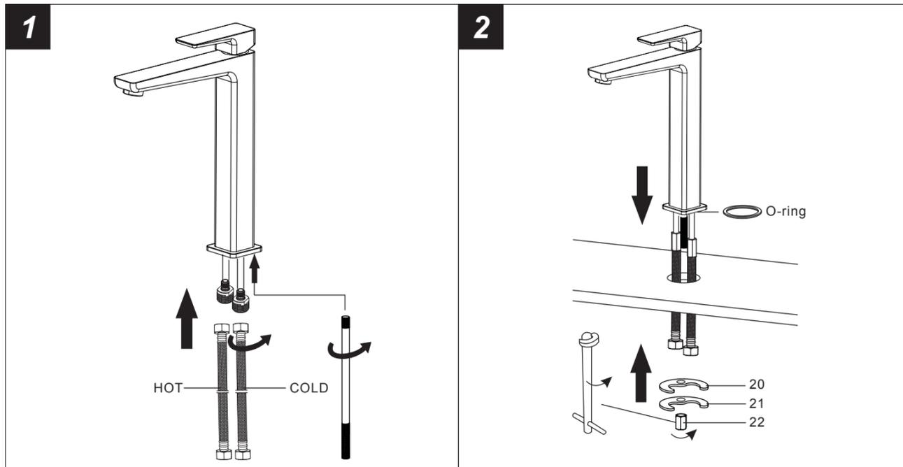
1. Assemble the 2 flexible hose and screw to the faucet by hand.
