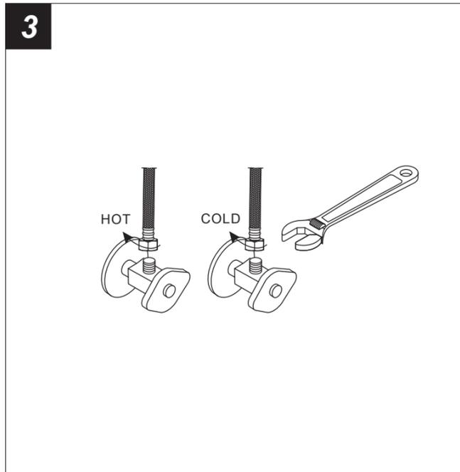
3. Connect the flexible hose to water supply valve (not included), and tighten it with adjustable wrench.
