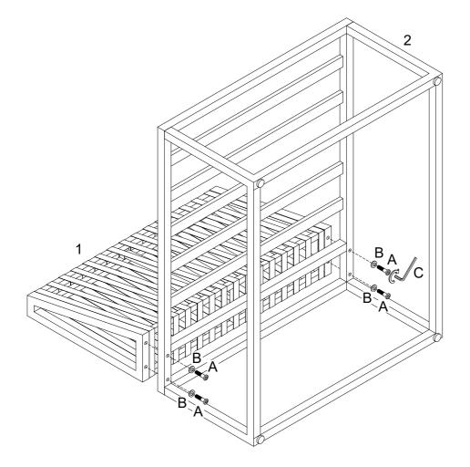
Using flat washer (B) and bolt (A) to attach part (2) to part (1) with hex key (C) as per diagram.
