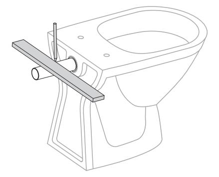
3. Carefully measure between your marks, this distance will be cut off the bald end. Add <sup>15</sup>/<sub>64</sub>" to measurement before cutting, leaving a small cushion for error.
