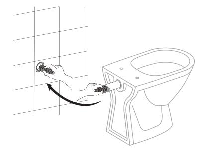
6. Ensure the bowl is level and install. Caulk and seal around the bowl.
