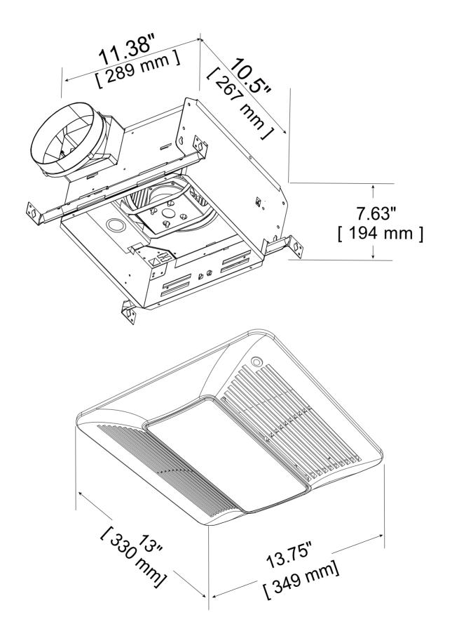
This fan can be installed to 11.5" - 24" between the joist or to I-joists, standard joists and truss construction.
