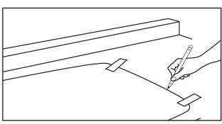
Draw a line parallel to the front edge of the countertop, indicating how far back the sink should be located. Typically the setback is 2" to 2-1/2" from the front of the counter, depending on the countertop overhang, the type of sink bowl and the size of the sink deck.
