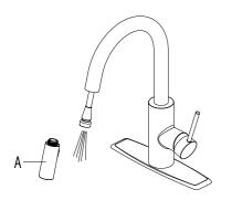
**NOTE**: Please make sure washer is installed attaching sprayer to hose.
