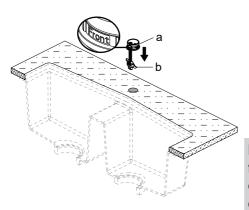
Shut off the water supply. Remove the old faucet. Clean the mounting surface. Check for the proper thickness of the sink. Insert the base (a) into sink. If your model does have a escutcheon, skip to step 1 b.
