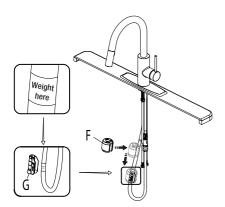
Install the weight clip (G) at the point of the hose marking "weight here". Insert the weight (F) onto the weight clip (G) by sliding it down onto the weight clip (G).
