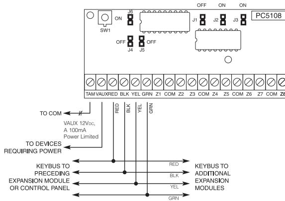
**TAM** - Used to tamper the cabinet in which the PC5108 is mounted. Connect a normally closed (NC) switch across TAM and BLK. If the tamper is not being used connect a piece of wire across TAM and BLK to remove the trouble condition.
