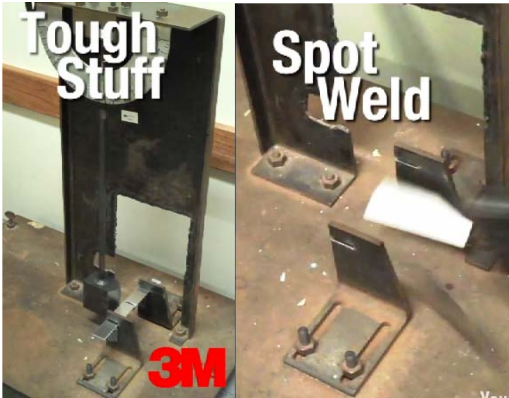
Figure 5. Toughened epoxy bond vs. spot welded bond, T6061 aluminum, pendulum impact test (3 lb weight on a 20" swing arm) http://www.youtube.com/watch?v=CPR28olqf5Y
