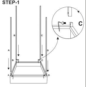
Secure All 4 Legs as shown considering marking ABCD with help of Allen Screws approx 50%.
