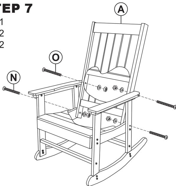
**TIP:** Insert all bolts before installing washers and nuts.
