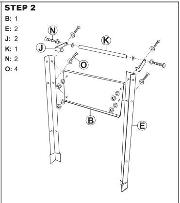
Do not fully tighten hardware until step 5 is complete.
