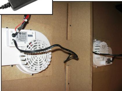
Two securely mounted turbo blade blowers, AC120V 60 Hz 0.31A, with a min. 9" x 12" mounting boards.
