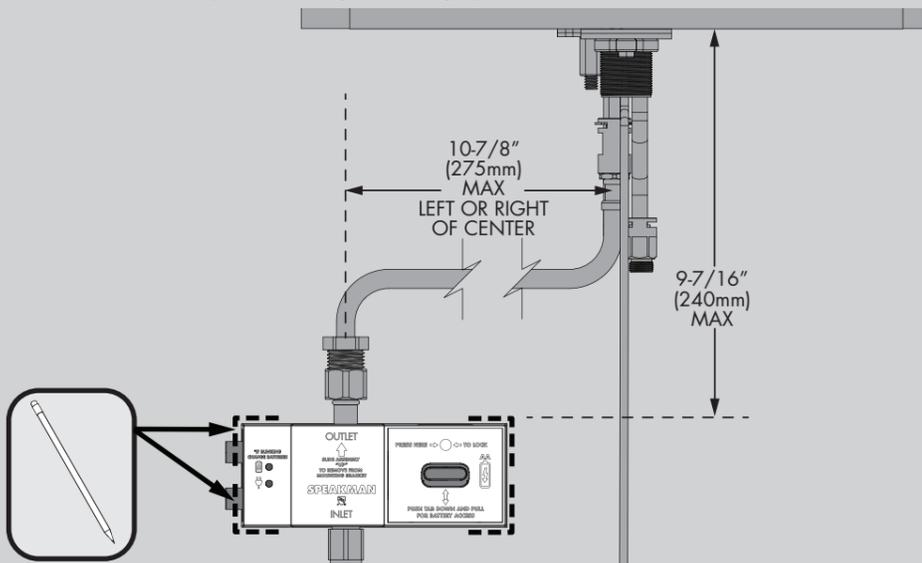
**7** Remove Mounting Bracket (1) from Solenoid Assembly. Using the previously marked location on mounting surface, align Mounting Bracket (1) horizontally to approximate position and mark the mounting locations with a pencil. If mounting on drywall and not to stud, use the appropriate anchors and fasteners for application. Recommend screw in easy anchor or equal for drywall.
