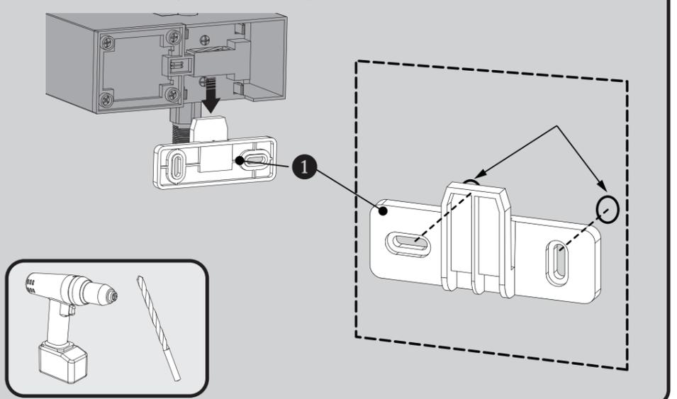
**8** After securing the Bracket to the mounting surface, align and slide Solenoid Assembly over Mounting Bracket.
