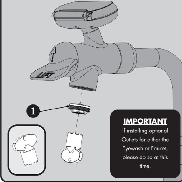
**16** Activate Faucet and test for proper operation. **NOTE: Before testing, you must remove tape from Eyewash Dust Cap.** Lift Eyewash Handle to activate Eyewash and test for proper operation. See "EYEWASH FLOW DATA" chart. Check all connections for leaks.
