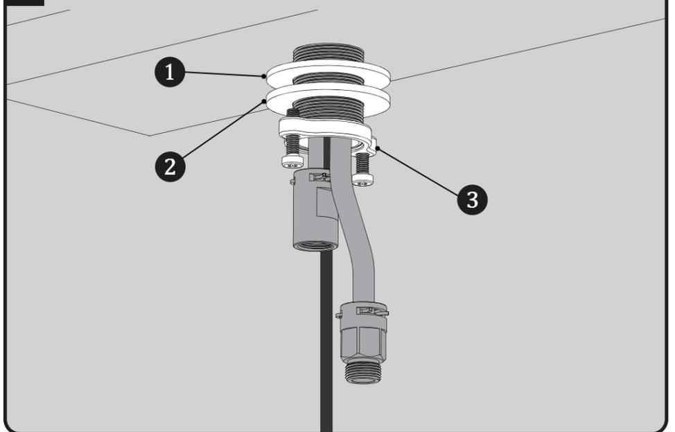
**3** This Faucet has a integral swivel feature. Verify sweep of Faucet Spout and align properly before securing Faucet Spout into final position.
