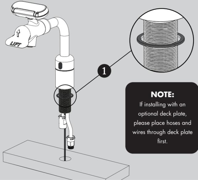
**2** From below, install Rubber Mounting Washer (1), Metal Mounting Washer (2), and Mounting Nut (3).
