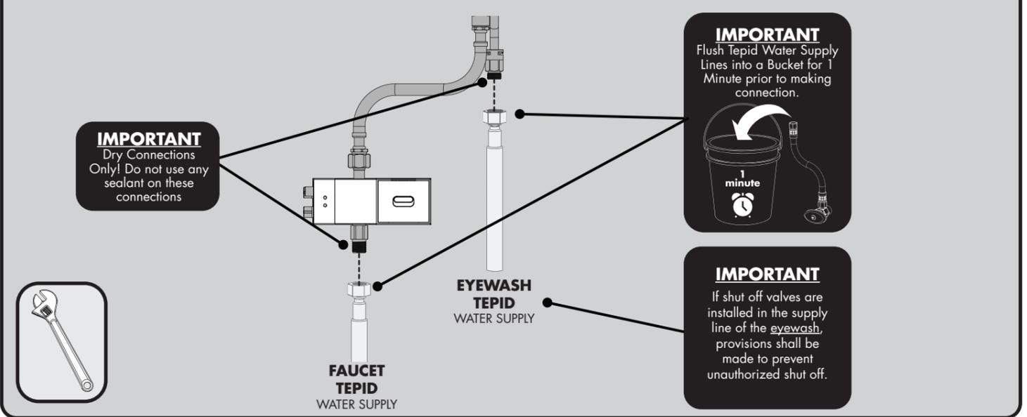
**14** After the assembly is complete, turn the Faucet and Eyewash water supplies on. Activate Sensor and allow Faucet to run for 1 minute to flush out any debris. Check all connections for leaks.
