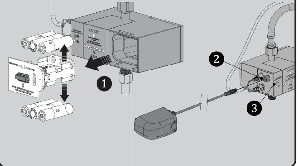
**12** Reinstall the Battery Tray (1). Make sure to press the indicated location until the battery door is fully seated and locks into position (2).
