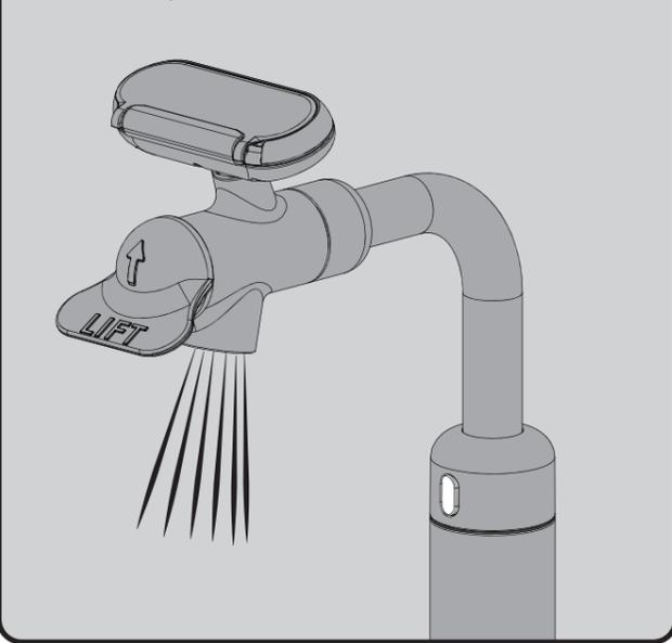
**15** Install Aerator (1) into the Faucet Outlet. Secure with included Aerator Wrench.
