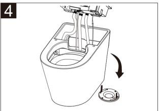
Install the toilet to the flange and ensure that the bolts are aligned with the holes in the toilet.
