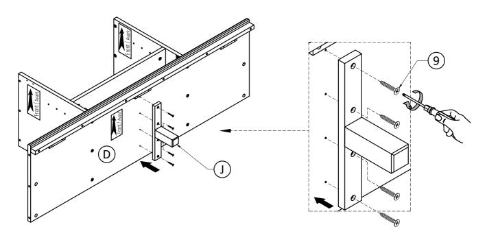
3. Align Bottom Support Leg ① with pre-drilled holes on back of Bottom Shelf ②. Use Phillips Screwdriver to tighten four Phillips Screws ②.
