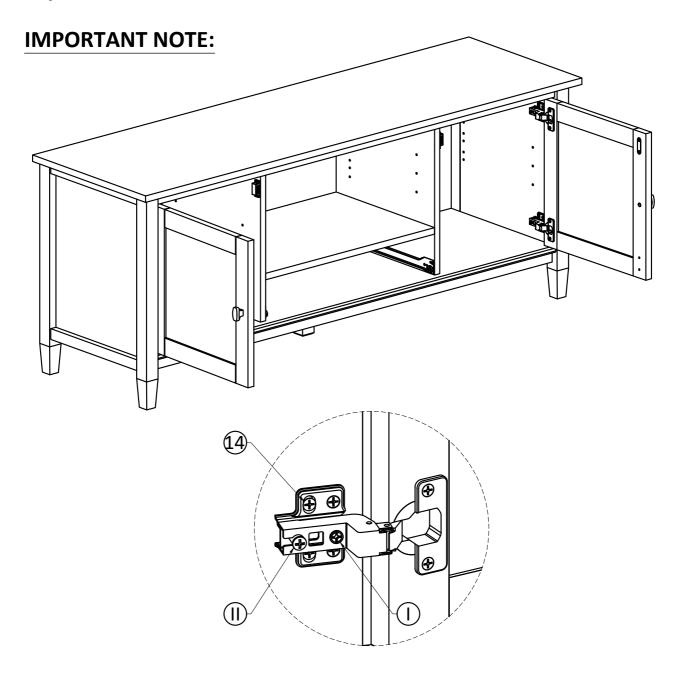
Tighten the Screw marked (I) to fasten hinge. The door may need to be adjusted so that all the spaces between the door and the unit sides are equal. To adjust, follow instructions:
