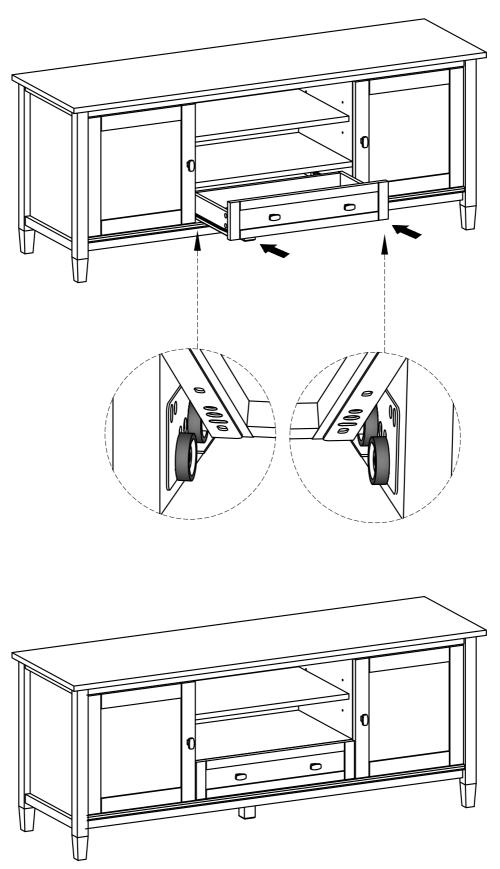
1. Insert assembled drawer into glides on assembled TV.
