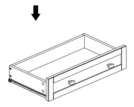
1. Use Phillips screwdriver to attach Handles 8 to Drawer Front K.
