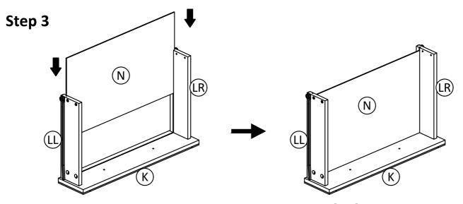
1. Slide Drawer Bottom (N) firmly into slots on Drawer Sides (L), (R) and Drawer Front (K).
