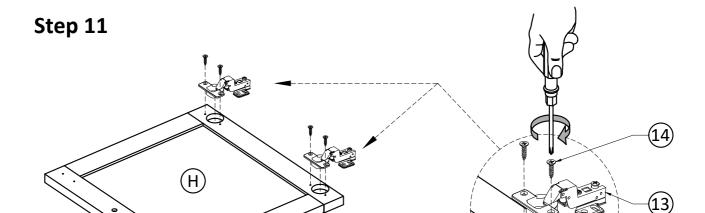
1. Attach Adjustable Hinges (13) to Doors (H) using Phillips Screws (14) into pre-drilled holes on Doors (H).
