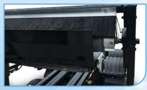
Optional trash brush closes the gap between stabilizer bar and tarp roller.
