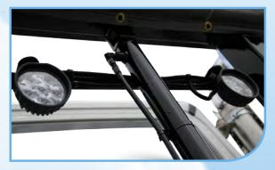
Gantry comes standard with light mounting brackets and a tube to run electrical wiring through for the lights.
