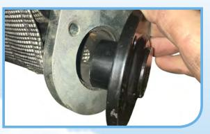
Tarp anchor tube cap with inner shaft extension enhances safety by preventing the tarp anchor tube from pulling out of the roll rest.
