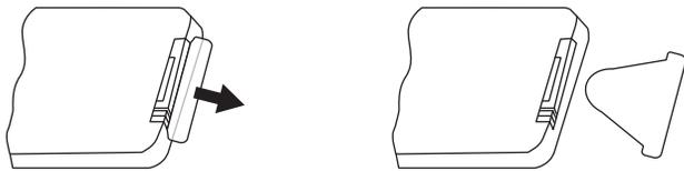
Pull the insulating film out of the battery cover before using the remote control.
