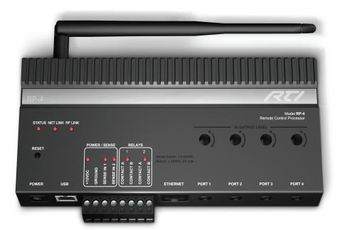
The RP-4 Control Processor is a powerful central controller that is designed for reliable control of audio/ video and other electronic systems. It combines an integrated 433MHz RF receiver, four assignable IR ports, relays, support for the RTiPanel App (ver 1.2 or higher) and more — all in a small, cost-effective package. The RP-4 is the perfect control processor for single room installations such as home theaters, media centers, and bedrooms.
