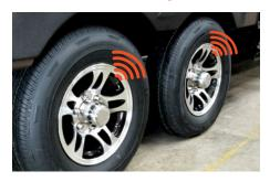
Sensors update pressure and temperature several times each minute while your RV is moving and check every 15 minutes while parked. Notifications sent any time the tires inflate, deflate or in the case of a blowout
