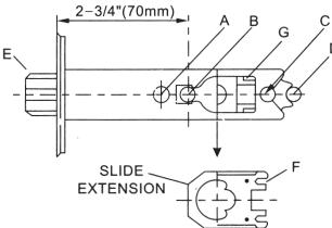
Note: To reverse the adjustment from 2-3/4"(70mm) to 2-3/8"(60mm):
