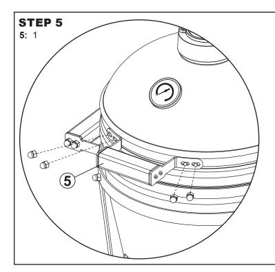
Remove the cap nuts from the threaded posts on the grill lid. Install Grill Handle (5) over the threaded posts and use the cap nuts to firmly secure it.
