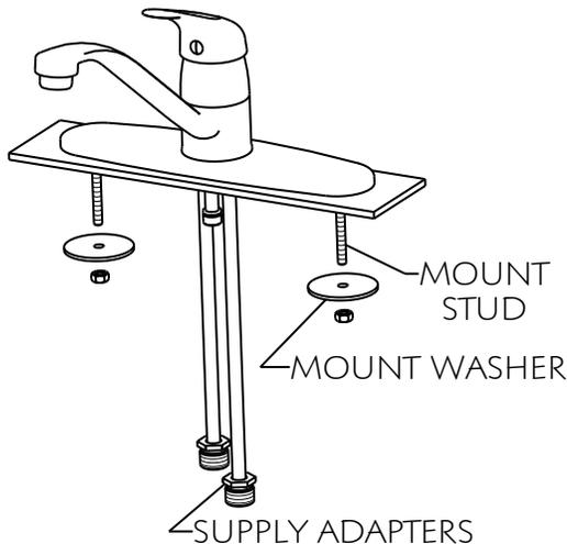
(MUST HOLD EACH ADAPTER HEX WITH WRENCH WHILE CONNECTING SUPPLIES.)
