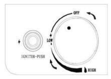
A. Press and hold the Electric Ignitor. Meanwhile, push and turn the Control Knob counter-clockwise to the "LOW" position. Keep pushing the Control Knob to light the burner.
