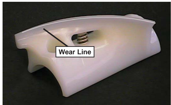
Figure 3-3 Auger Flight Wear
