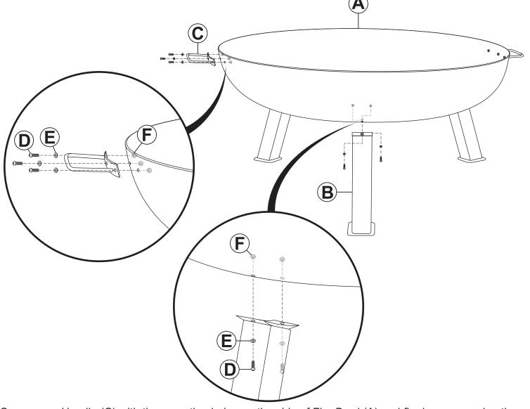
Secure one Handle (C) with the mounting holes on the side of Fire Bowl (A) and firmly secure using three Bolts (D), three Washers (E) and three Nuts (F). Repeat to secure the remaining handle.
