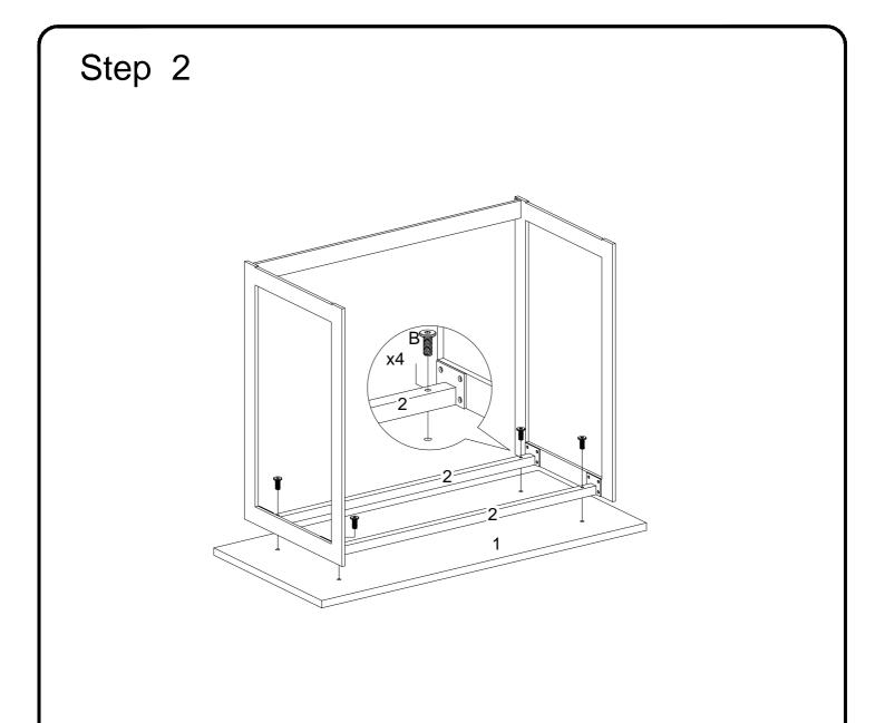
Attach part (3, 4) to part (1) using bolt (B) with hey key (C).
