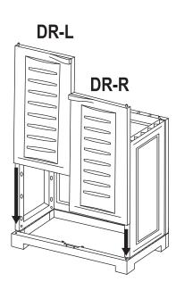
Ensuring the handles are at the top, align the pivot pins on the bottom of Left Door (DR-L) and Right Door (DR-R) with the bottom panel.
