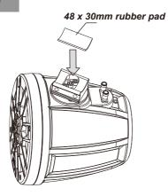
Place a supplied rubber (48 x 30 mm) pad on the metal base of the mounting band to prevent abrasion and secure clamping.
