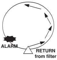
If the water returning from the filter is positioned at 6 oíclock and the flow is counterclockwise, the best location to put the alarm is between 8 oíclock to 9 oíclock position.
