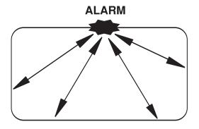
Place alarm in a central location for shortest distance from all parts of the pool
