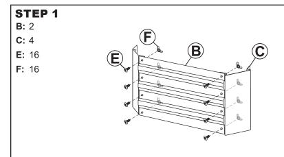
**IMPORTANT:** Identify the rolled edges of the panels and ensure they are installed facing the inside of the garden bed.
