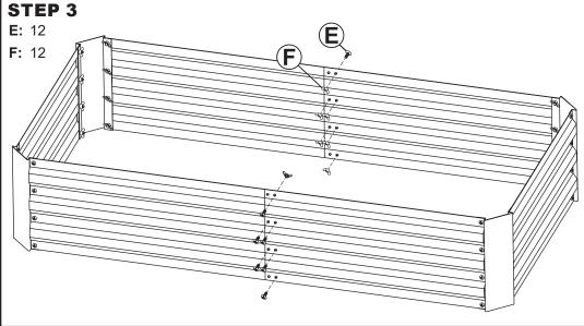
**IMPORTANT:** The location of hardware installation in the diagram is for maximum stability of the unit, the center bar must be installed in the correct location to achieve optimal structural support.
