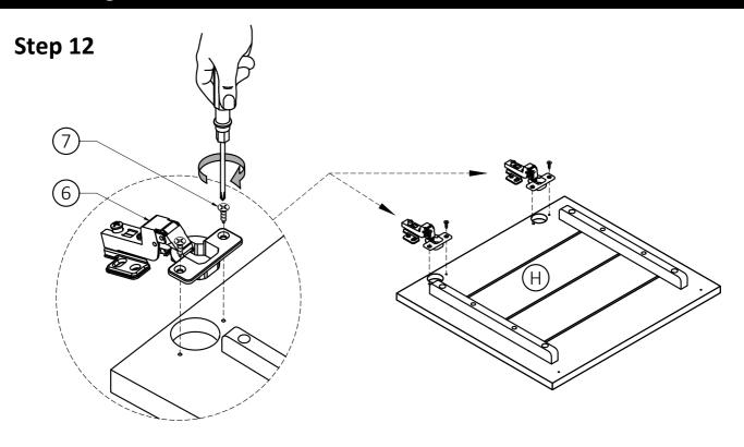
1. Attach Adjustable Hinges 6 to Doors H using Phillips Screws 7 into pre-drilled holes on Doors H.
