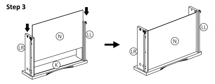
1. Slide Drawer Bottom (N) firmly into slots on Drawer Sides (L), (R) and Drawer Front (S).
