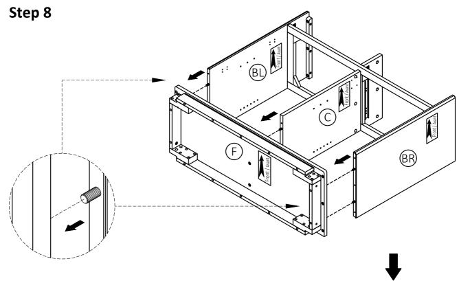
1. Align Wood Dowels with guide holes and attach Sides (BL), (BR) and Divider (C) to Bottom (F).
