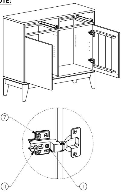
Tighten the Screw marked (I) to fasten hinge. The door may need to be adjusted so that all the spaces between the door and the unit sides are equal. To adjust, follow instructions:
