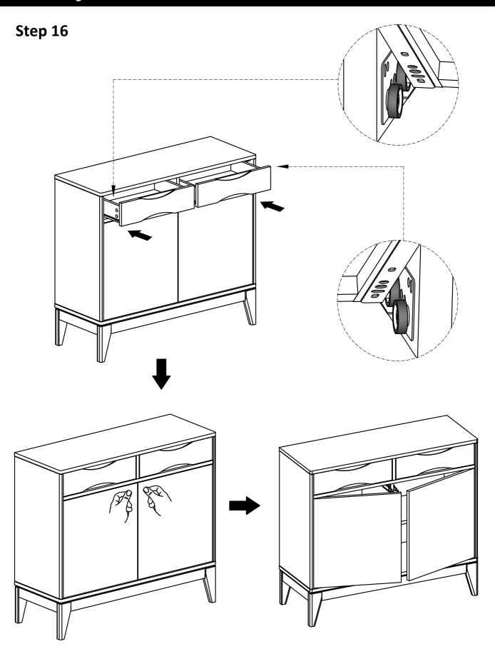
1. Insert assembled drawers into glides on assembled cabinet.
