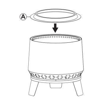
Place Heat Deflector (A) onto the inner liner.
