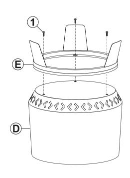
Align Base (E) with the bottom of Fire Bowl (D) and secure using three M6x12mm Bolts (1).
