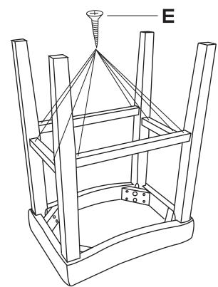
Using your own screwdriver 100% lock Self-tapping Screw (E) as shown in the diagram
