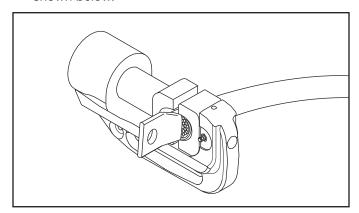
For a UL or cUL classified crimp, complete the number of crimps specified under "Connector Selection". 4. For a single crimp, position the connector so the crimp will be located at the center of the barrel.
