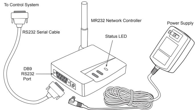
The MR232 Protocol Guide provides more information about how to configure command sequences to pass from a building automation control system through the MR232 Network Controller and on to the Miro wireless system. Instructions for installation, binding operations, and use are included with the relevant wireless devices. Application support information and installation guides are available online.
