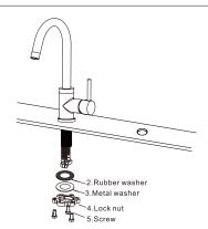
2. Adjust the position of the faucet and secure it with the fixing kit as photo.
