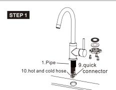
1.Position the faucet, o-ring on the installation surface. And then put the faucet into center hole.
