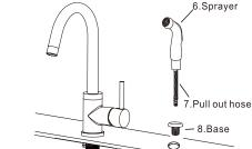
3. Put the base into the hole. Put the sprayer and pull out hose through the base. secure it with the fixing kit as photo.
