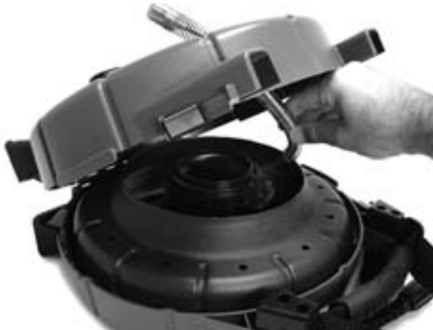
Figure 5 – Routing The Camera Head
