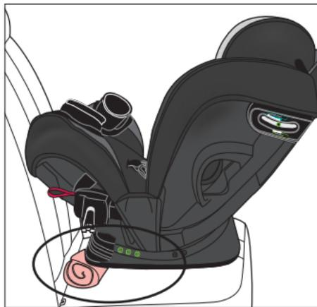
**Note:** In some vehicles, in **Position 1**, it may be necessary to place a tightly rolled towel or small blanket beneath the front edge of the child restraint to provide enough recline so that the leveling ball is in the green zone for rear-facing use.
