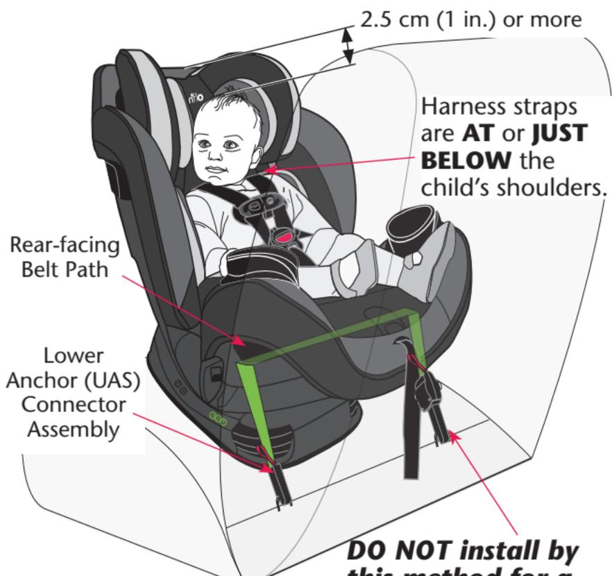
**DO NOT install by this method for a child weighing more than 18kg (40lbs).**
