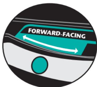
Re-check the level indicator. Ball should be between the blue zone for forward-facing.
