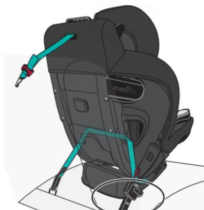
Tighten the strap by moving the handle back and forth on the lower anchor connector as shown until the seat is tight. Fold handle up after tightening.
