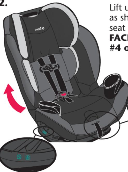
Lift up on the recline lever as shown and adjust the seat recline to **FORWARD-FACING Recline Positions #4 or #5 ONLY.**
