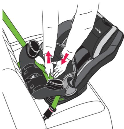
**The vehicle seat belt must be as tight as possible.** Using your full weight, push the child restraint firmly into the vehicle seat as you tighten the vehicle **seat belt**, as shown. Reconnect the seat pad to the front of the child restraint.
