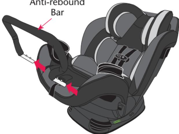
To remove the Anti-rebound Bar, press both locking buttons and withdraw the Bar from the seat.
