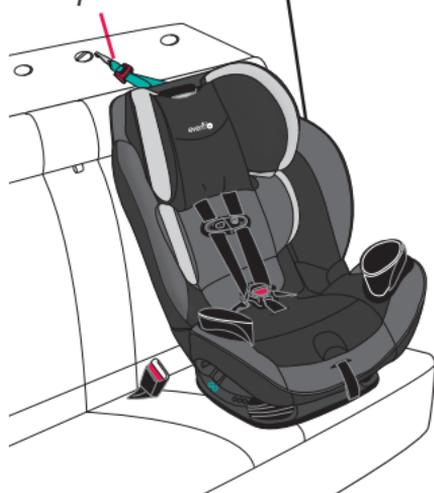
Place child restraint in your vehicle **forward-facing**, as shown. Always make sure the bottom of the child restraint sits flat on the vehicle seat.
