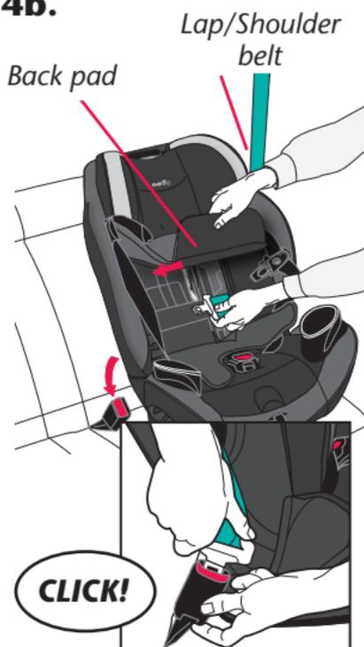
Raise headrest to its highest position (p. 58), then lift back pad away from child restraint for easier access. Route the lap/shoulder belt through the forward-facing belt path and continue through the opposite opening of the child restraint. Fasten the buckle.
