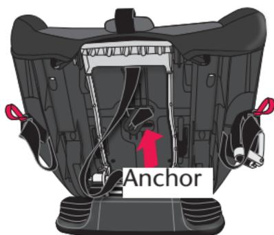
Remove the crotch buckle from the crotch slot. Recline the seat to **Recline Position 1** and turn the anchor and push it up through slot in the seat. Pull crotch buckle off seat.
