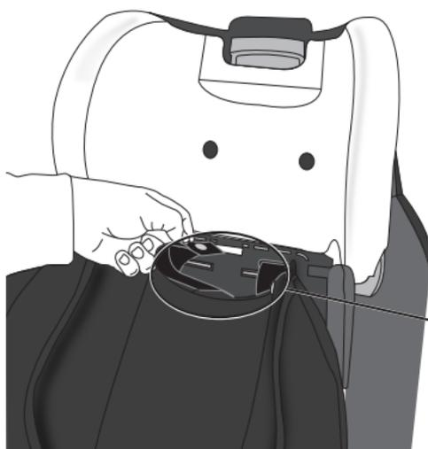
Pull the strap out of the opening in the head support board.
