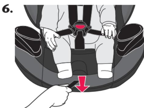
Hold the chest clip while pulling the harness adjustment strap so that the chest clip does not ride up into the child's neck. The harness straps must be snug against the child. A snug strap should not allow any slack. It lies in a relatively straight line without sagging. It does not press on the child's flesh or push the child's body into an unnatural position.
