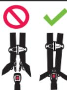
Children have **STRANGLLED** in loose or partially buckled harness straps. Fully restrain the child even when carrier is used outside the vehicle.
