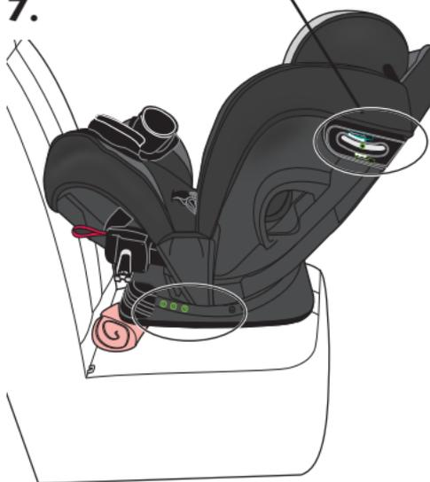
**Note:** In some vehicles, in the most reclined position, it may be necessary to place a tightly rolled towel or small blanket beneath the front edge of the child restraint to provide enough recline so that the leveling ball is in the green zone for rear-facing use.
