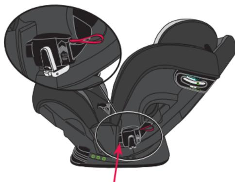
Rear-facing **lower anchor (UAS)** storage compartment\*
