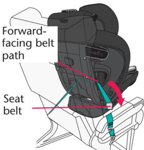
Adjust the child restraint to **Recline Position #5** (p. 58), then place it on the aircraft seat **forward-facing**.
