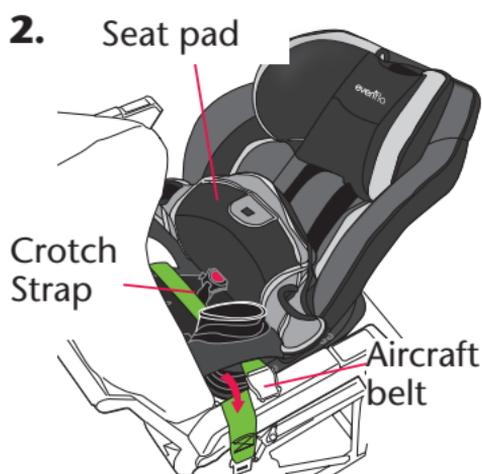
Pull the seat pad off the front of the child restraint. Route the aircraft seat belt through the rear-facing belt path opening on one side and continue through the belt path opening on the opposite side of the child restraint, as shown above.
