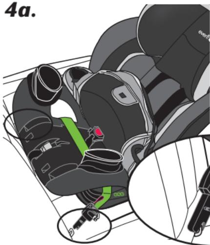
Lift pad off front edge of seat as shown.
