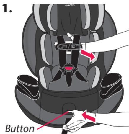
Push the harness release button on the front of the seat. At the same time, pull on the harness straps.
