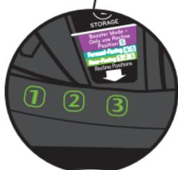
To raise or lower the recline, pull the handle out in front edge of seat and push or pull seat into the desired recline position as shown.
