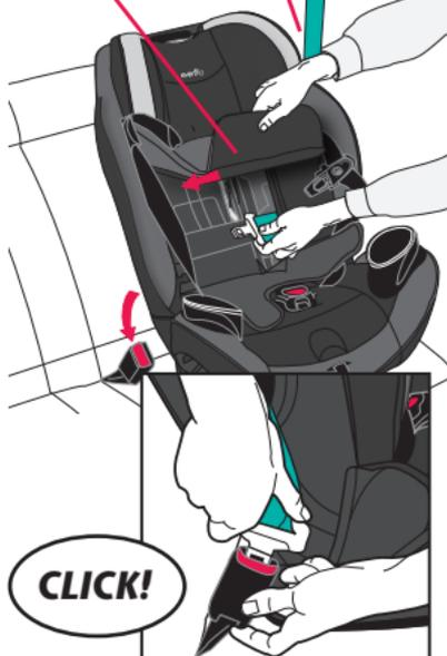
Raise headrest to its highest position (p. 58), then lift back pad away from child restraint for easier access. Route the lap/shoulder belt through the forward-facing belt path and continue through the opposite opening of the child restraint. Fasten the buckle.
