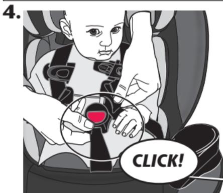
Insert both buckle tongues into the buckle. Pull up on the harness strap to check that the buckle tongues are fastened and to remove any slack from the webbing around the child's legs.
