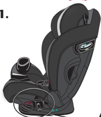
Re-route the lower anchor connector strap through the rear-facing belt path (p. 28). Store the lower anchor connector (UAS) in the rear-facing belt path as shown.
