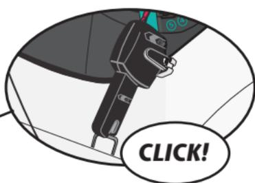
**IMPORTANT:** Make sure both lower anchor connectors are facing upward and the straps are not twisted.
