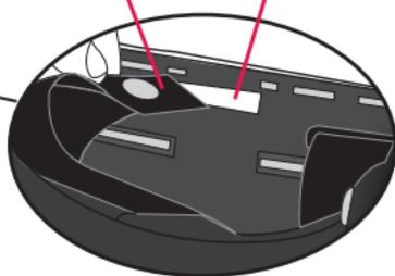
7. To remove headrest pad, lower backrest flap and slide pocket off headrest.
