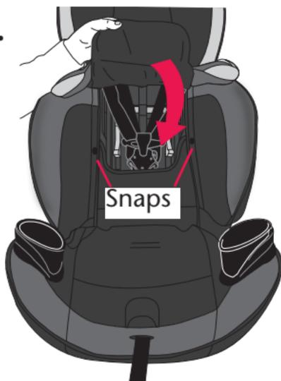
Raise back pad and fasten the two snaps on side of seat pad then lower the headrest pad.
