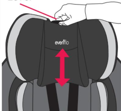
To adjust, squeeze the headrest adjust lever, as shown, while sliding the headrest up or down to the desired position. When the headrest is in one of the locking positions, the adjust lever will pop into its original position.
