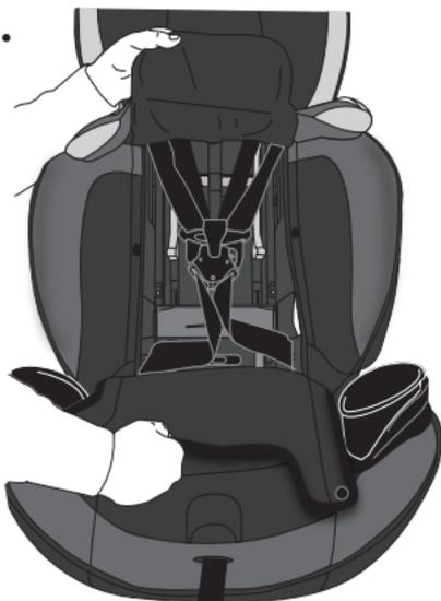
Reassemble the loose crotch buckle onto the shoulder straps and fasten the chest clip.
