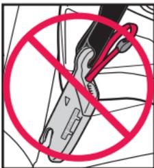
**IMPORTANT:** Make sure both lower anchor connectors are facing upward and the straps are not twisted.
