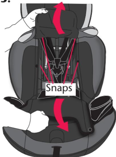
Unfasten two snaps at the harness slot openings where the shoulder straps come out then unfasten snaps on the inside of the seating area. Pull the back pad forward.
