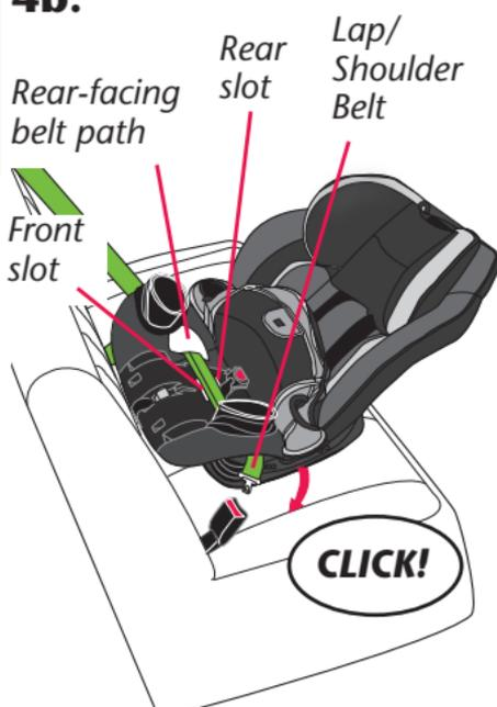
Pull the seat pad off of the front of the child restraint. Route the lap/shoulder belt through the rear-facing belt path and continue through the opposite opening of the child restraint. Fasten the buckle.
