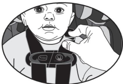
Check the harness straps near the shoulders for slack. You should **NOT** be able to pinch the harness (see illustration). Adjust as needed.
