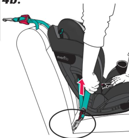
Attach lower anchor / UAS connectors to the vehicle lower anchor bars until they lock onto the bars on both sides of the seat.
