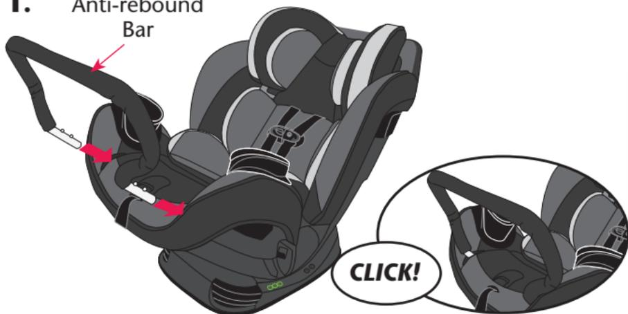
Place Anti-rebound Bar through slots in seat cover into metal tubing in seat shell.
