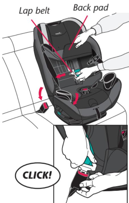
Raise headrest to its highest position (p. 58), then lift back pad away from child restraint for easier access. Route the lap belt through the forward-facing belt path and continue through the opposite opening of the child restraint. Fasten the buckle.
