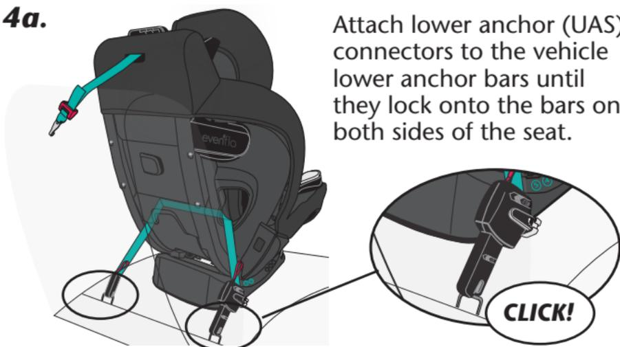
**IMPORTANT:** Make sure both lower anchor connectors are facing upward and the straps are not twisted.
