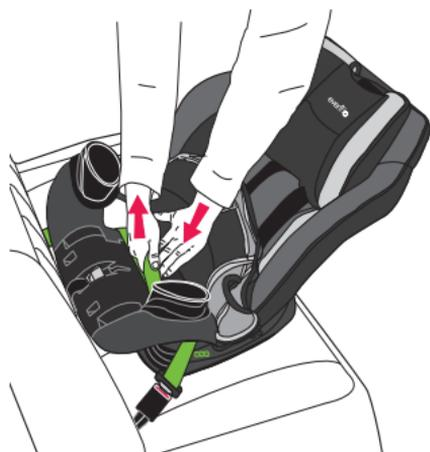
**The vehicle seat belt must be as tight as possible.**
