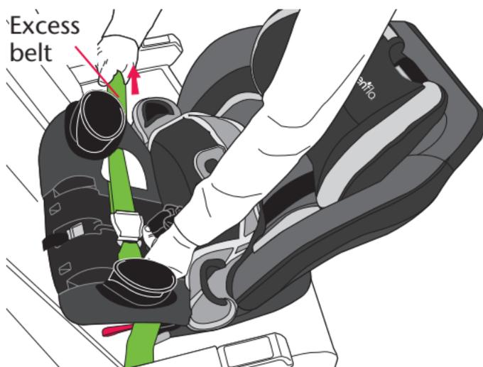
The aircraft seat belt must be as tight as possible. Route the excess seat belt strap back through the rear-facing belt path opening, as shown above. Using your full weight, push the child restraint firmly onto the aircraft seat while pulling on the excess seat belt strap to tighten.
