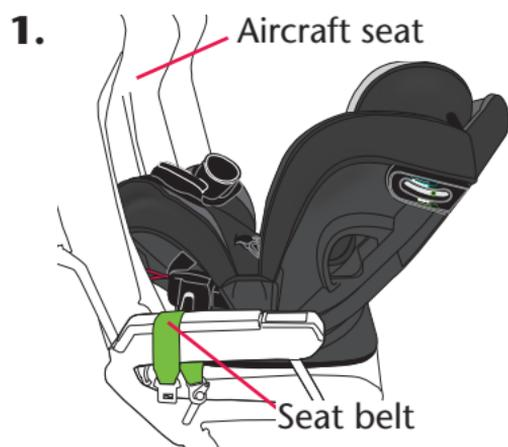
Unbuckle the aircraft seat belts and lay over the armrests, as shown. Adjust the child restraint to its **Recline Position 1, 2 or 3** (p. 58), then place it on the aircraft seat **rear-facing**.
