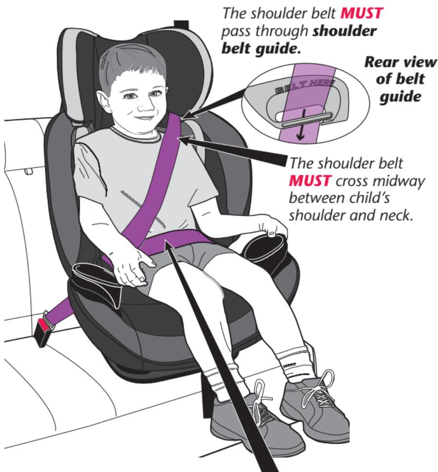
*The lap belt is stretched low and snug across the child's hips, within the lower belt guides, and fastened into the buckle.*
