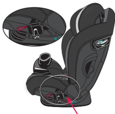
Forward-facing **lower anchor (UAS)** storage compartment\*
