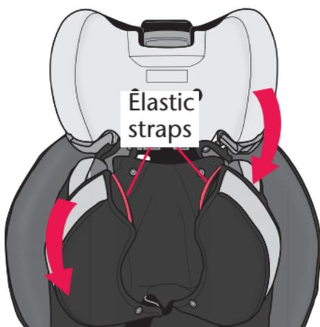
Slide headrest pad over headrest and remove the elastic straps around the vehicle belt guides.
