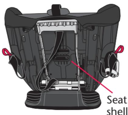
To reposition the crotch strap, first recline the seat to Recline Position #1 (p. 58). Looking under the front of the seat, turn the crotch strap harness anchor sideways and push it through the slot in the bottom of the seat shell. Reposition the crotch strap into the other slot. Make certain the crotch strap is properly seated against the seat shell.
