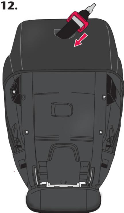
Unclip tether from the tether anchor bar and push through slot in seat pad as shown.
