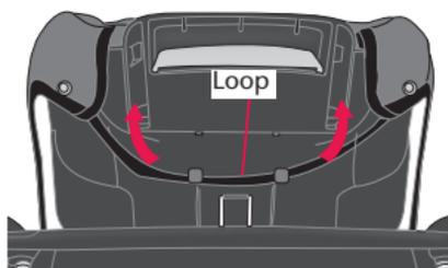
Remove elastic straps from around the vehicle belt guides.
