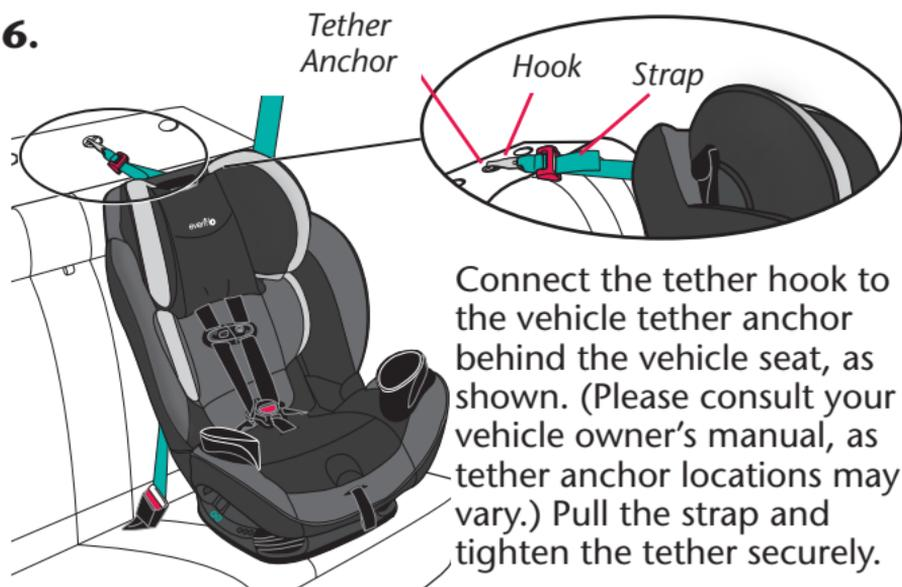
Connect the tether hook to the vehicle tether anchor behind the vehicle seat, as shown. (Please consult your vehicle owner's manual, as tether anchor locations may vary.) Pull the strap and tighten the tether securely.
