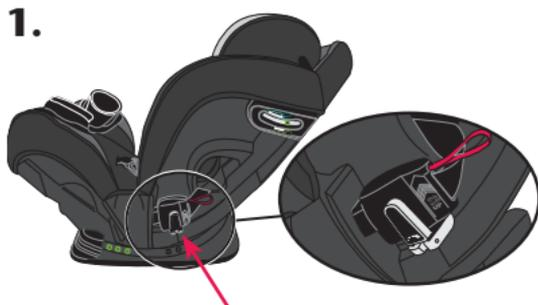
Rear-facing **lower anchor (UAS)** storage compartment
