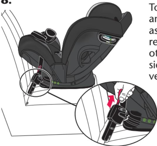
To remove the lower anchor connector assembly strap, pull red release strap. Remove the other strap on the other side of the seat from the vehicle anchor.
