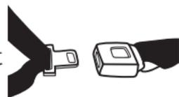
Check vehicle owner's manual for specific instructions. The vehicle belt is tightened after switching the retractor by pulling up on shoulder belt and feeding the webbing into the retractor.
