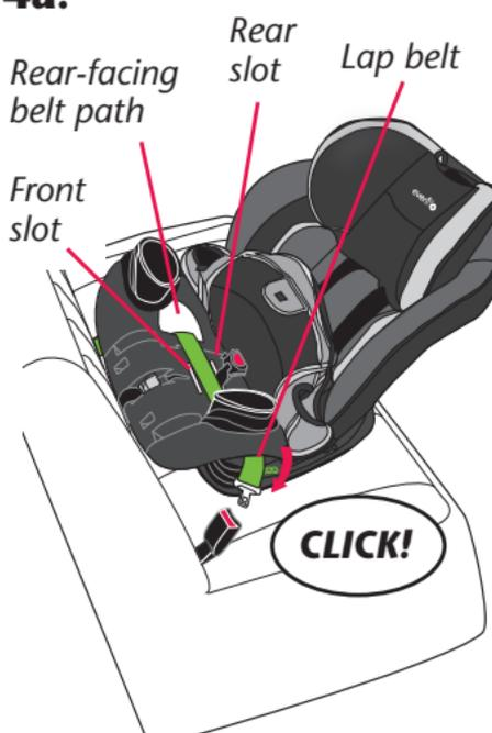
Pull the seat pad off of the front of the child restraint. Route the lap belt through the rear-facing belt path and continue through the opposite opening of the child restraint. Fasten the buckle.
