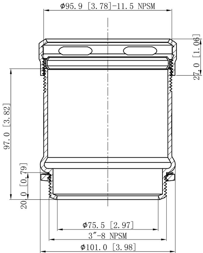
CUTAWAY VIEW A-A
