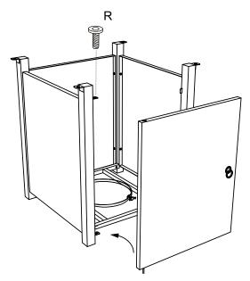
Step3. Hang the bottom (H) of the door plate on the round bracket. Top with 1PC screw(R)lock.
