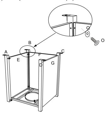
Step2. Connect panel (E,F,G)with table legs(A,B,C,D) by 12pcs screws (O) and 12pcs M6 washers(Q).
