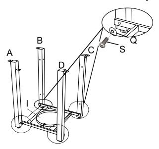
Step1.Connect the tank holder/base (I) With table Lets(A/B/C/D) by 4pcs screws (S)and 4pcs M6 washers(Q).
