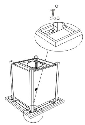
Step4.Attach the assembled base to the bottom of top using 4pcs of screws (O),and 4pcs M6 washers(Q), make sure the panel (L) faces the valve stem. Tighten all screws.
