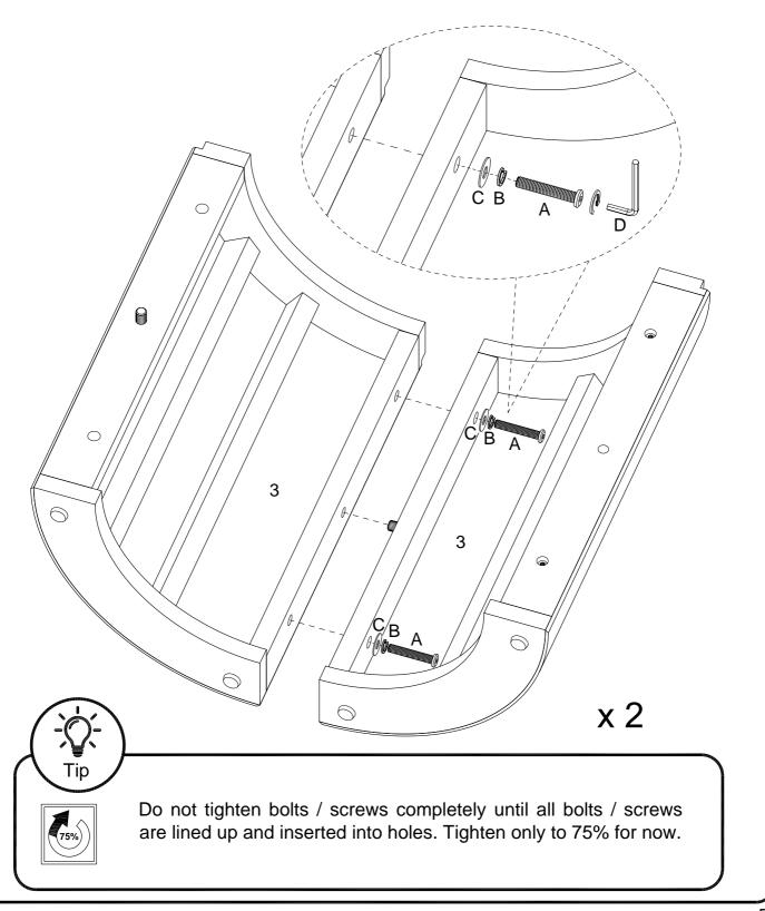
Time to bring it all together! Join both halves using the same Washer (C), Spring Washer (B), and Bolts (A). Tighten everything up with the hex key (D).
