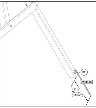
Warning! To prevent tipping and avoid potential injury, stakes must be driven 13"(330mm) into ground. Digging or driving stakes can be dangerous if you do not check first for under-ground wiring, cables or gas lines.
