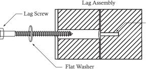
Before mounting Lag Screw, use factory drilled holes as guides to drill 1/8" (3.2mm) pilot holes
