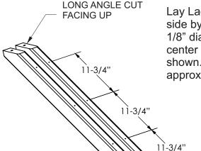
Lay Ladder Rails (PG-24-0031) side by side. Mark and drill four 1/8" diameter holes along the center of each rail at locations shown. Holes should be approximately 1/4" deep.
