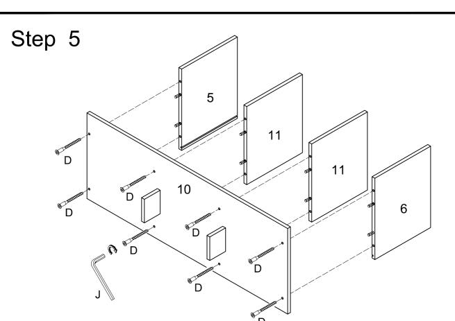
Secure dividers (5,6,11) to bottom panel (10) using bolts (D) as shown in the diagram.
