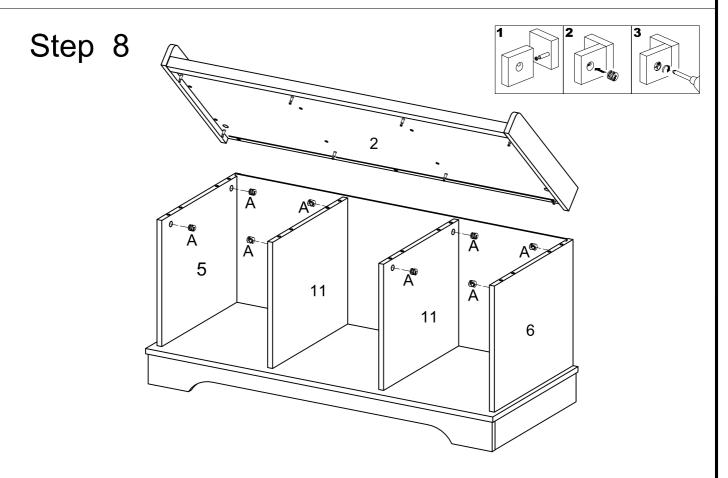
Place top assembly onto lower frame as shown in the diagram. Insert cam locks (A) as shown and tighten using a screwdriver.
