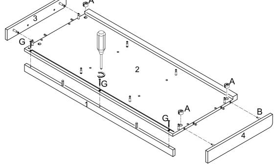
Attach parts (1,3,4) to part (2) as shown in the diagram. Carefully place cam locks (A) into part (2) and tighten using a screwdriver.
