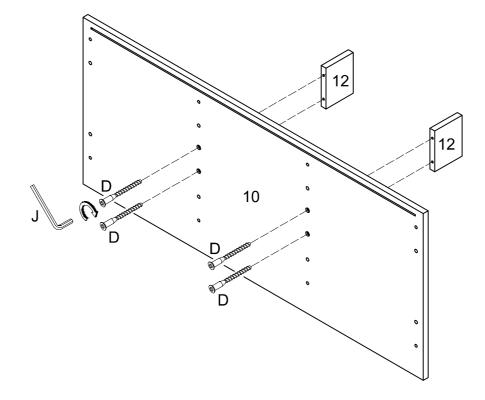
Secure supports (12) to bottom panel (10) using bolts (D) as shown in the diagram.
