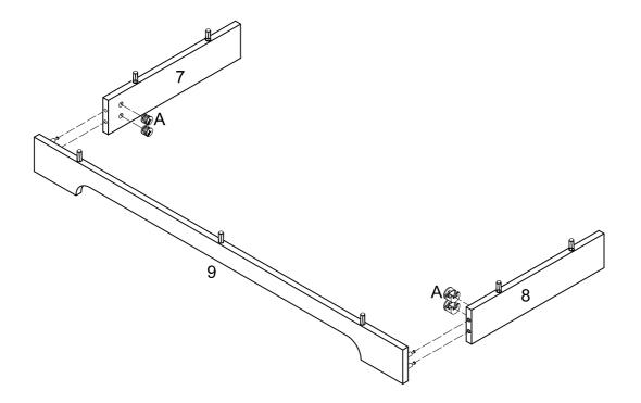
Attach parts (7,8) to part (9) as shown in the diagram. Carefully place cam locks (A) into parts (7,8) and tighten using a screwdriver.
