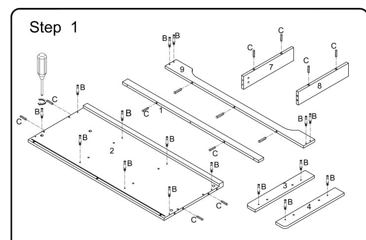
Inserts dowels (C) into parts (1,2,7,8,9) and screw cam bolts (B) into parts (2,3,4,9) as shown in the diagram.
