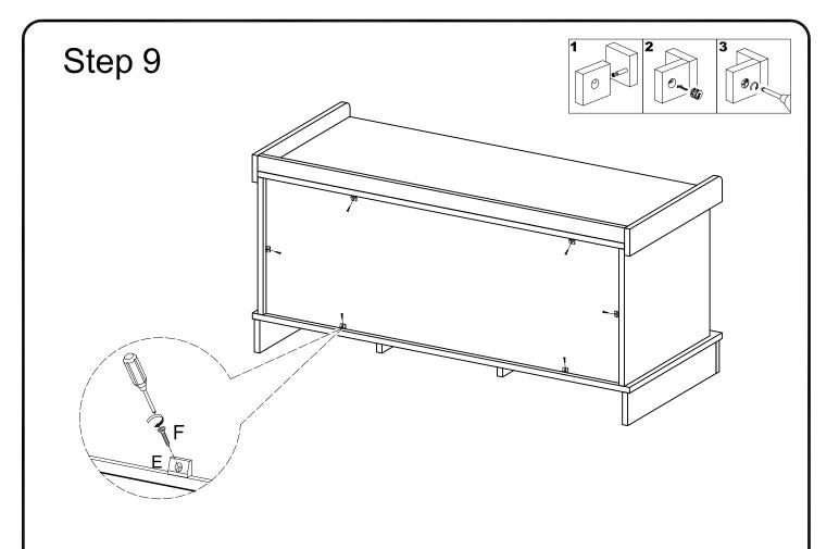
Insert wedges (E) to the back panel and secure using screws (F) as shown in the diagram.
