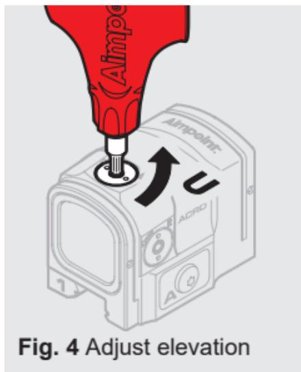
**Fig. 4** Adjust elevation
