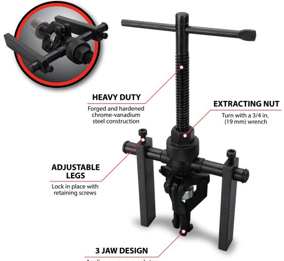
Applies pressure evenly to prevent damage to the bearing
