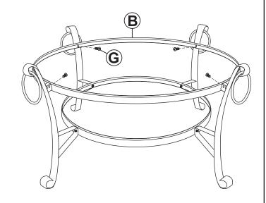
Align Top Ring (B) with the tops of the legs and loosely secure by hand-tightening four M6 Bolts (G). Fully tighten all bolts on the top and bottom rings.
