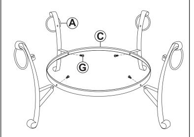
Loosely secure four Legs (A) to Bottom Ring (C) by hand-tightening four M6 Bolts (G).
