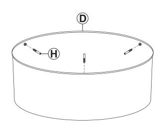
Install three M8 Grub Screws (H) to the inside rim of Fire Bowl (D).
