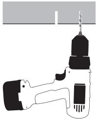
Select a suitable drill bit an drill pilot holes.
