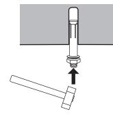
If installing into concrete/brick, tap in the expansion bolts. Expand them enough to hold in place by tightening the nuts, *do not fully tighten yet!*
